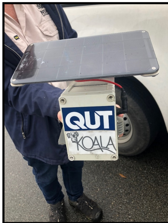
A KOALA unit measuring air quality, one is installed at Cammeraygal HS Senior Campus. There are 10 in total.
